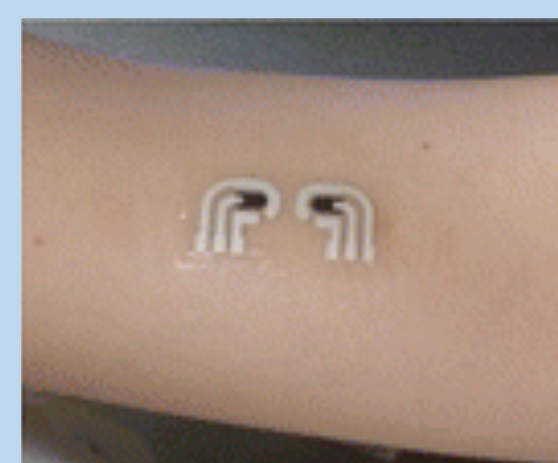
Figure 3. Tattoo-based monitoring sensor (Bandodkar, 2014).
