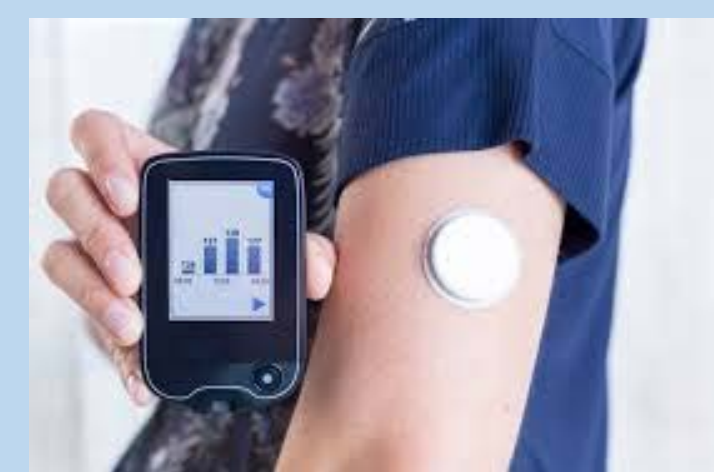
Figure 2. Continuous glucose monitor patch with a needle inserting into the arm. Tracks changes in blood sugar (time.com).
